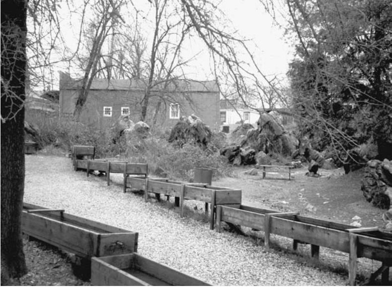
Long toms, like these near the miner's cabin in Columbia, were used for recovering gold from placer deposits during the gold rush.
